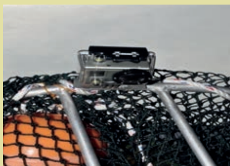
Photo 2: Underwater camera fitted to TED
