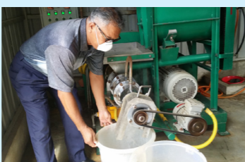
A trainer processing aquafeed using an extruder during Farm-made Feed Training Course at FRI Pulau Sayak, Kedah.
