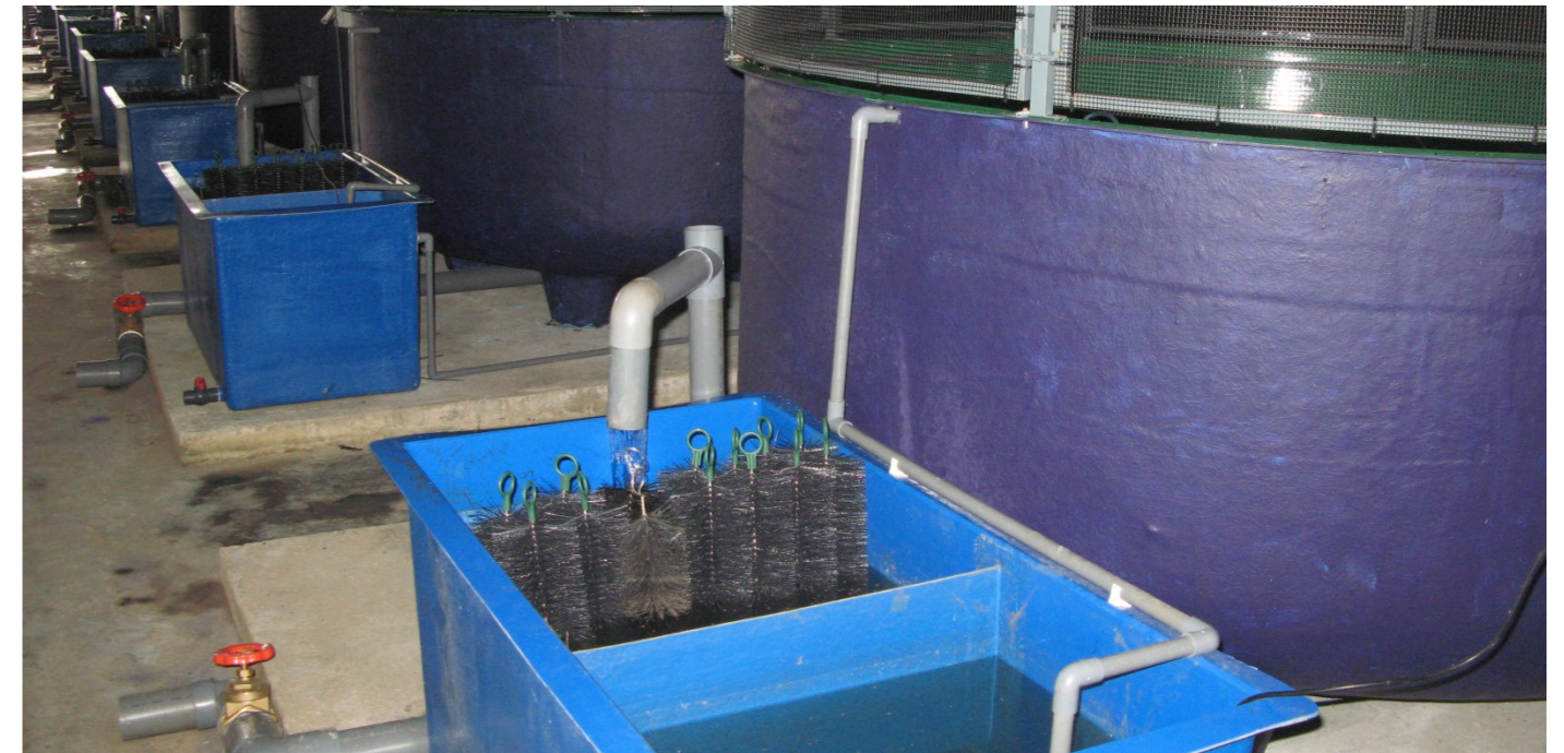
The domesticated Kelah brooders were stocked in the FRI Glami Lemi's own developed 5MT RAS tanks
