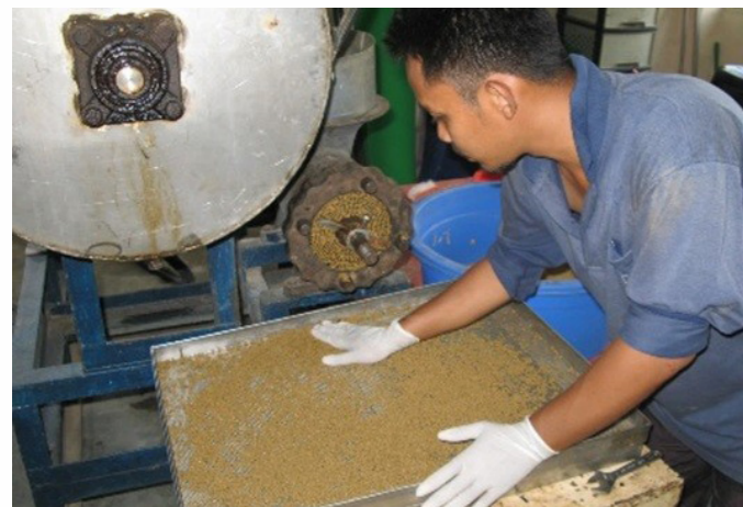
Processing maturation diet using 'Mini Pelleting Machine'
