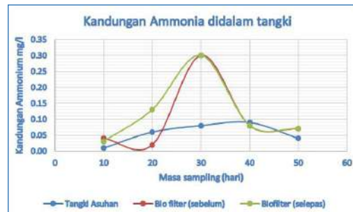
Kandungan Amonium didalam tangki asuhan dan biofilter sebelum dan selepas air dirawat. Ammonium content in the nursing tank and biofilter before and after treatment
