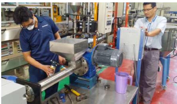
Pengujian inverter prototaip kedua mesin ekstruder Experimenting the inverter of the second prototype extruder machine
