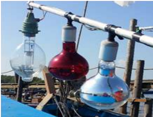
Mentol lampu (Metal Halide) yang digunakan Light bulbs that were used to attract squids
