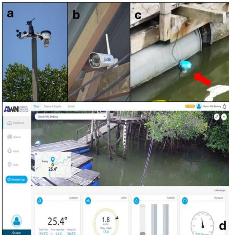
Figure 2: Installation overview of various IoT devices and the internet homepage screen that records them. (a) Weather meter, (b) weather camera, (c) water temperature buoy (arrow), and (d) home page screen displaying live data (Yurimoto et al., 2025c).
