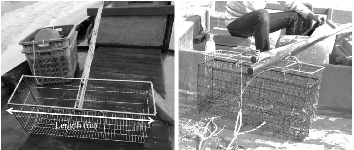
Figure 1. Two types of long dragged scoops with different mesh size were used in this study (left: coarse mesh size of 20 mm, right: fine mesh size of 5mm). The length of the long-dragged scoop opening was measured for density calculation
